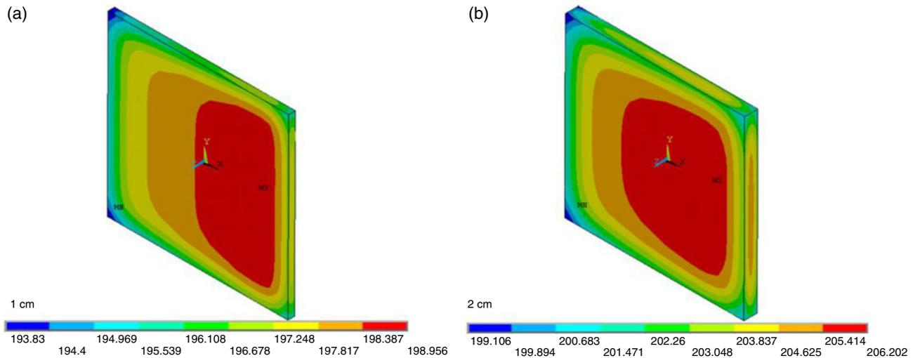
**Figure 1.** Temperature distribution of Yb:YAG: (a) temperature of 1 cm Yb:YAG; (b) temperature of 2 cm Yb:YAG.
