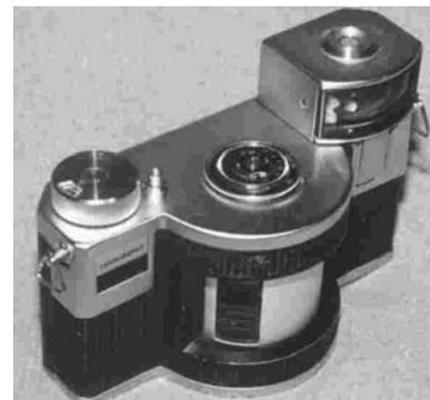
**Fig. 1.** The panoramic Horizont camera. The camera uses ordinary, 35 mm film, with a frame size of 24 mm × 58 mm. It has a 120° field of view and a theoretical focal length of 28 mm.
