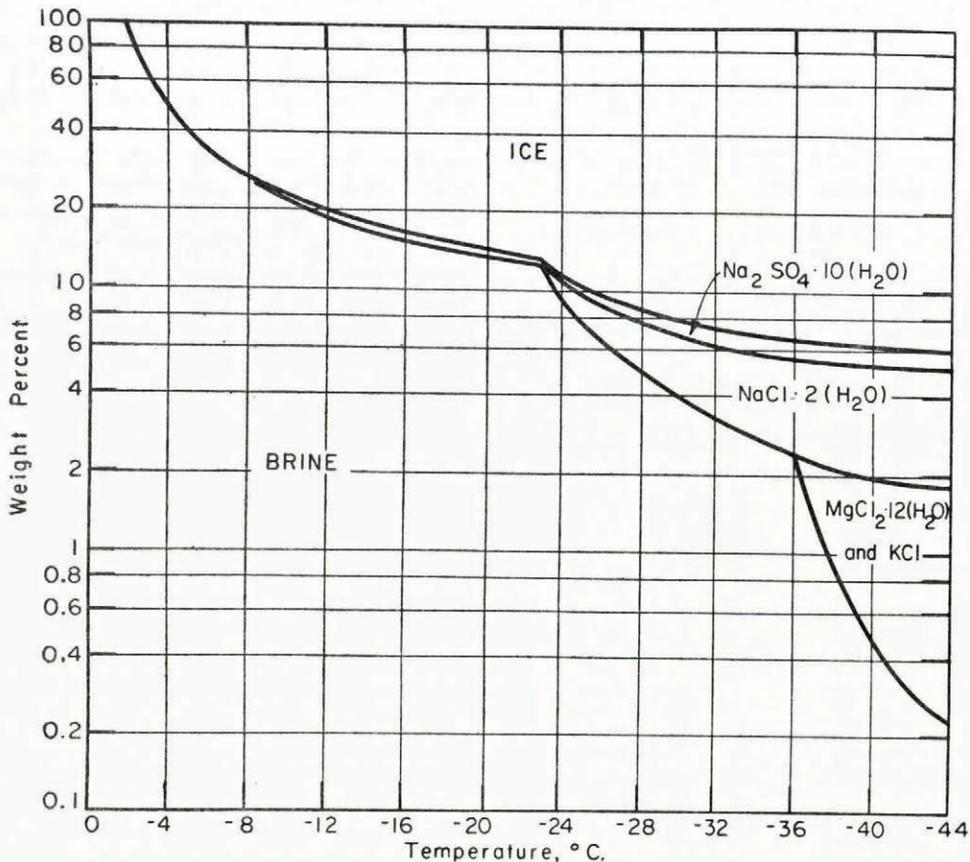
Fig. 2. Phase diagram in the solidification of sea-water. After D. Anderson<sup>14</sup> from data of K. H. Nelson and T. G. Thompson<sup>13</sup>
