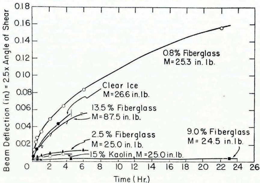
Fig. 1. Deformation of various samples in bend tests with bending moment  $M$  as indicated on curves. Slope of curves is a measure of apparent viscosity (1 in. lb. = 1.15 gm. cm.; 1 in. = 2.54 cm.)
