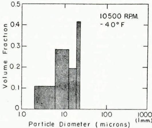
Fig. 4. Product of snow grinder with rotor speed of 10,500 r.p.m. at an ambient temperature of -40° F. (-40° C.)
