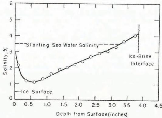
Fig. 3. Salinity versus thickness for freshly formed sea ice frozen 30 hours from a 9 in. (23 cm.) deep pool at -40° F. (-40° C.)
