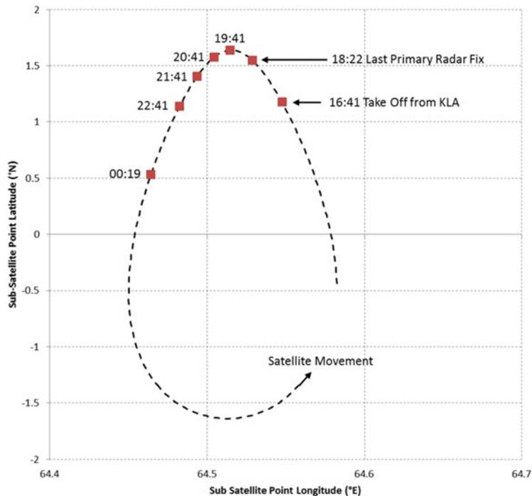
Figure 8. 3F1 Sub-Satellite Point Locations during MH370 Flight.
