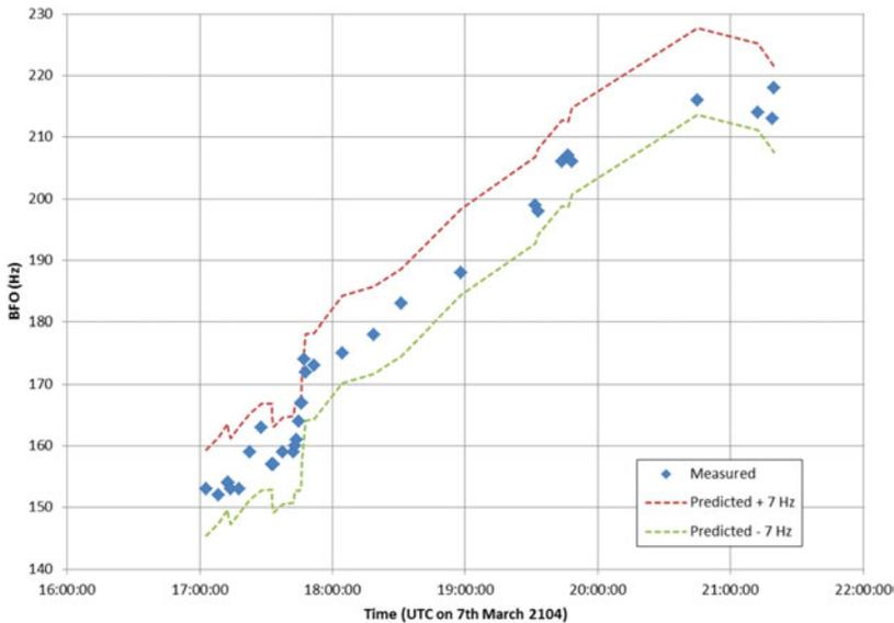
Figure 15. Burst Frequency Offset Validation (Amsterdam Flight).
