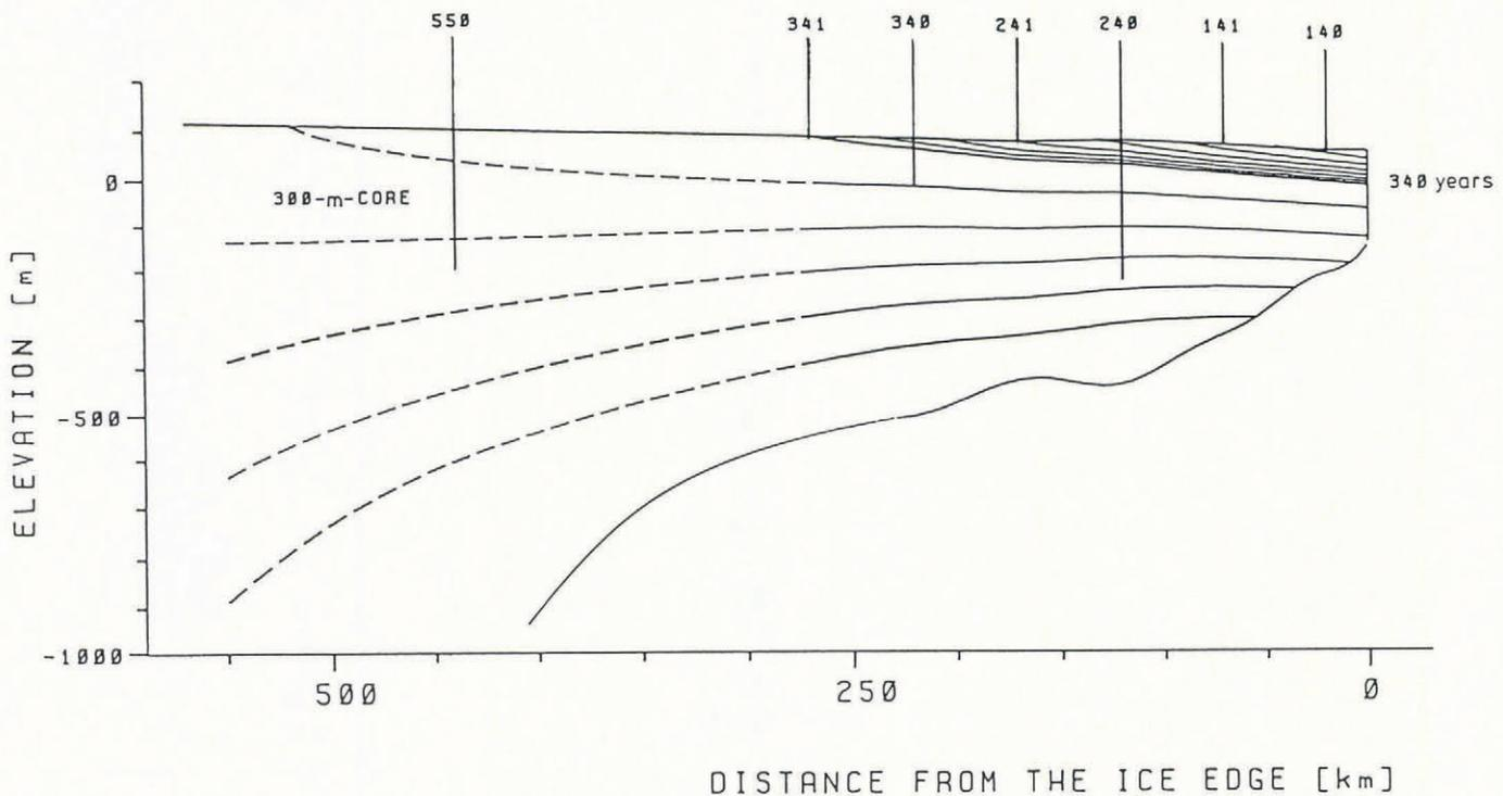
Fig.7. Particle paths in the Ronne Ice Shelf along a flow line through measuring point 340.
