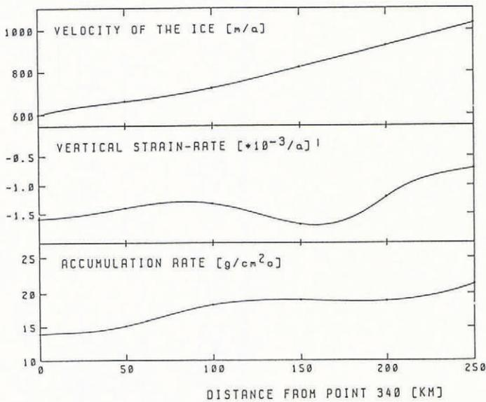
Fig.6. Parameters used to calculate the particle paths in the Ronne Ice Shelf along a flow line through the drilling site (measuring point 340 in Fig.1).
