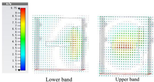
Fig. 5. Simulated surface current distribution of the unit.
