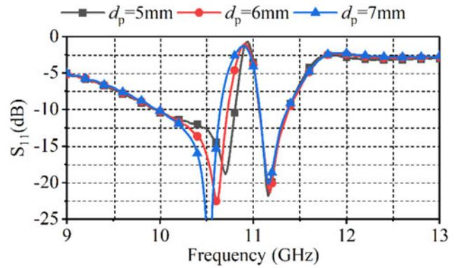
Fig. 10. Parametric analysis of the  $d_p$  of  $S_{11}$ .
