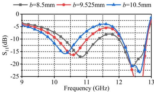
Fig. 9. Parametric analysis of the  $b$  of  $S_{11}$ .
