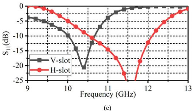
Fig. 2. (a) Model of horizontal polarization antenna; (b) the model of vertical polarization antenna; and (c) the simulated  $S_{11}$  ( $l_1 = 12$  mm,  $l_2 = 15$  mm).
