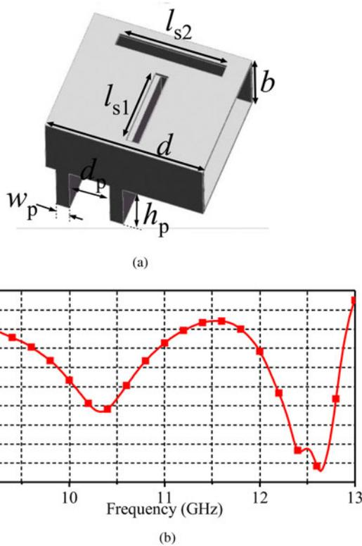
Fig. 8. (a) Model with two grooves at the bottom and (b) the  $S_{11}$  of the model.
