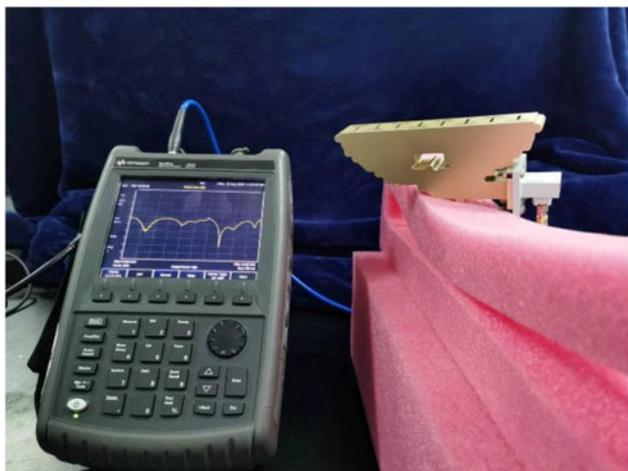
**Fig. 13.** Fabricated antenna.
