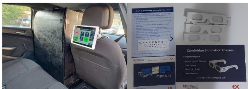
Figure 5. Used testing equipment, a wizard of oz AV (left) and simulation glasses (right)
