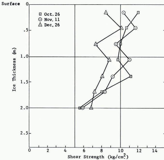
Fig. 6. Shear-strength profile of the sea-ice sheet on 26 October, 11 November and 26 December 1964
