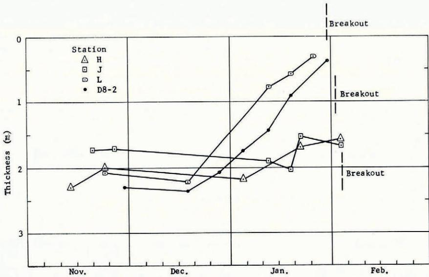
Fig. 11. Ice-thickness changes during the summer of "Deep Freeze 65". NCEL Cape Armitage stations D8-2, L, H and J
