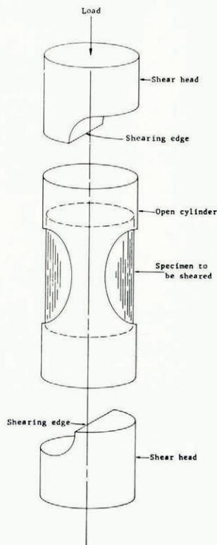
Fig. 2. Open cylinder shear apparatus
