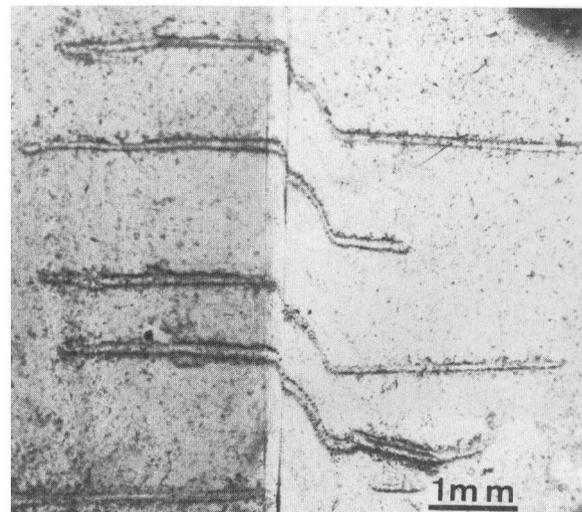
Fig. 3. Intense intragranular shear near a grain boundary.
