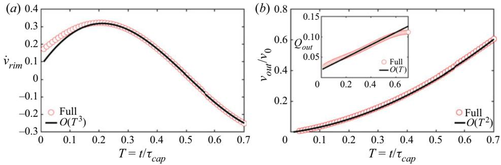
Figure 26. (a) Full prediction of the time evolution of the rate of change of rim’s volume  $\dot{V}_{rim}$ , compared with the approximate analytic expression (A9). (b) Full prediction of the time evolution of the volume rate,  $Q_{out}$ , (inset) and fraction of cumulative volume,  $V_{out}/V_0$ , shed from the rim, compared with their approximate analytic expressions (A11) and (A12).
