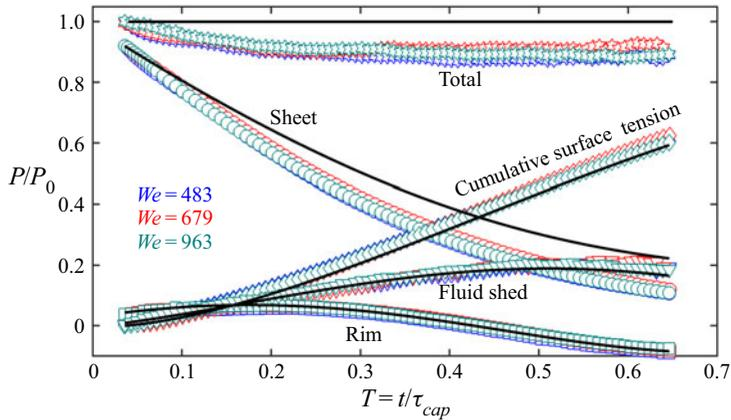
Figure 14. The partition of momentum fractions in each sub-part of the fluid system is independent of  $We$ . The small derivation of total momentum from unity originates from a second-order effect on the sheet dynamics at early time (as shown in figure 12b).
