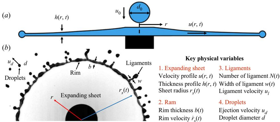
Figure 1. (a) Schematic diameter of canonical unsteady fragmentation upon drop impact on a rod of comparable size,  $d_r$ , to that of the impacting drop,  $d_0$ . (b) Snapshot of unsteady sheet upon drop impact on a rod with definition of key physical quantities of the fluid system involved.
