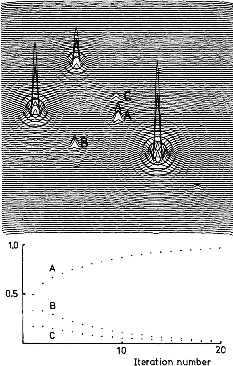
Fig 7. The use of a window technique on a field of 4 point sources. (a) Hybrid map (1st iteration) made from amplitudes (3 bright sources and source A), together with phases (3 bright sources). (b) Changes in the correct peak A and spurious peaks B and C in the hybrid map with successive iterations. The intensity scale is normalized to the correct value for peak A.
