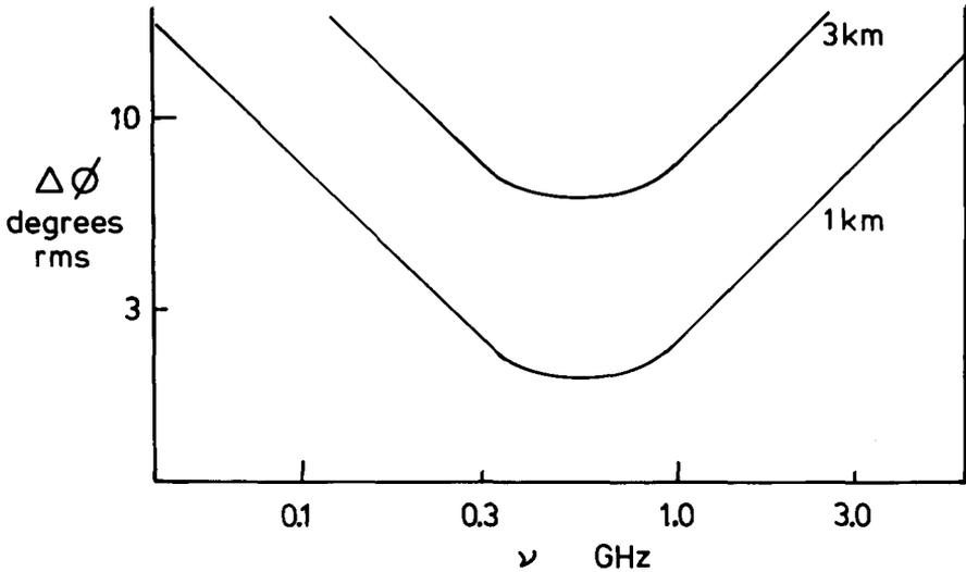
Fig 1. Typical rms phase variations due to ionospheric and tropospheric irregularities as a function of frequency and baseline.
