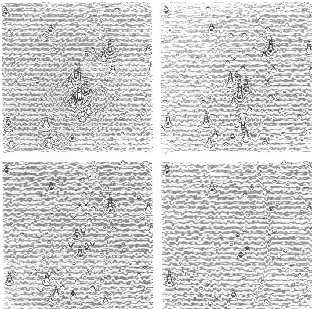
Fig 4. The effect of different trial distributions on the interpretation of hybrid maps. Difference maps made for a distribution of 10 point sources and trial distributions comprising successively 1, 2, 3 and 4 of the sources. Positions of 8 of the sources are marked by •, the remaining 2 lie outside the plotted area. The four sources of the trials are the central three and the upper right hand one. Notice that residual peaks at their positions gradually become smaller.
