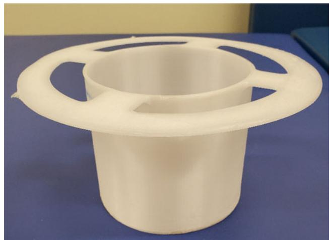
**Figure 3.** 3D-printed cylindrical phantom used to evaluate noise.
