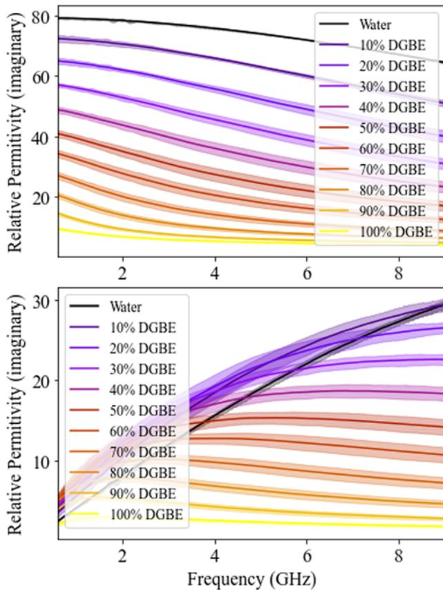
**Figure 4.** The real (top) and imaginary (bottom) relative permittivity of varying DGBE–water liquid solutions from 0.6 to 9 GHz.
