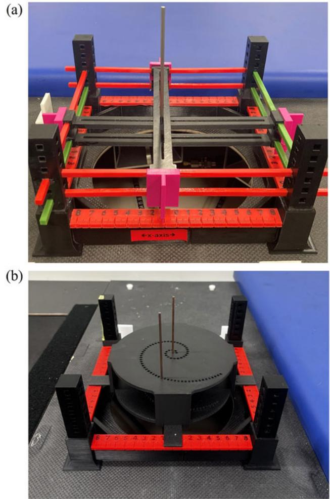
**Figure 2.** (a) Single-rod positioning system, and (b) dual-rod positioning system used to evaluate spatial resolution.
