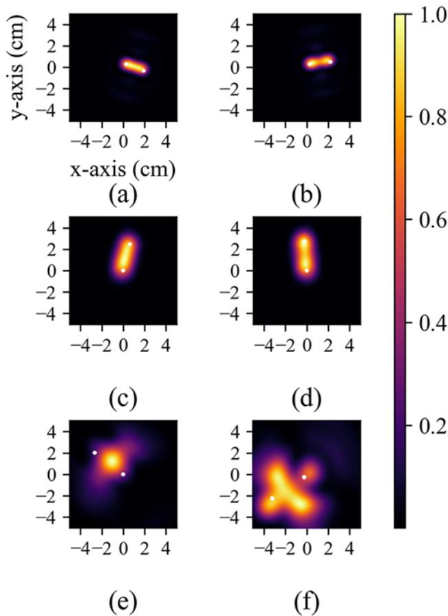
**Figure 6.** Two-target image analysis displaying indistinguishable (left) and distinguishable (right) targets of the bed system (a, b), bench-top system (c, d), and portable system (e, f).
