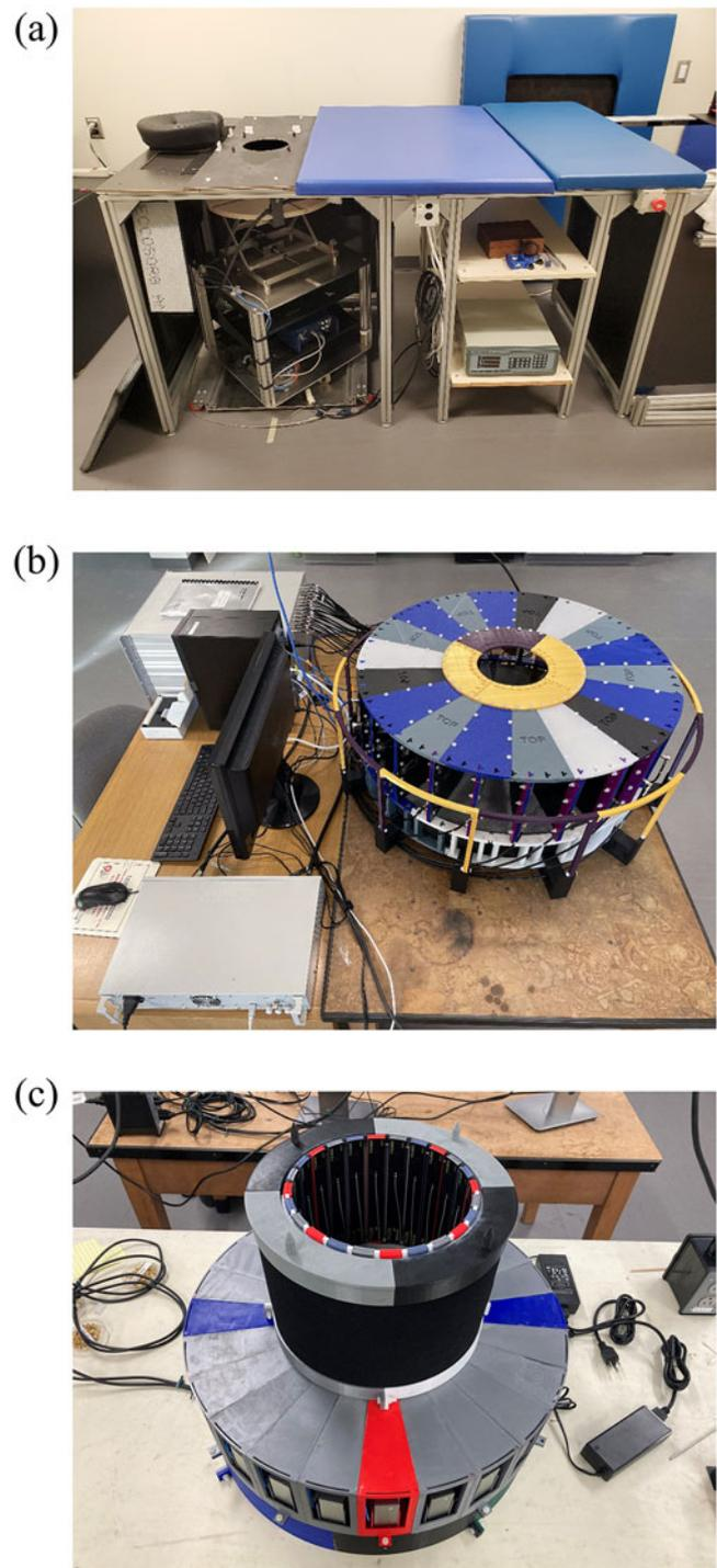
**Figure 1.** The three BMS used in this work: (a) Bed-based imaging system, (b) Bench-top system, and (c) Portable system.
