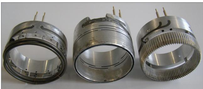
**Fig. 5.** Melting head with hotspring® coil heater of 100 mm outer diameter. Left: open heater; middle: simple aluminum heat spreader; right: aluminum crown with heat-spreader fins.
