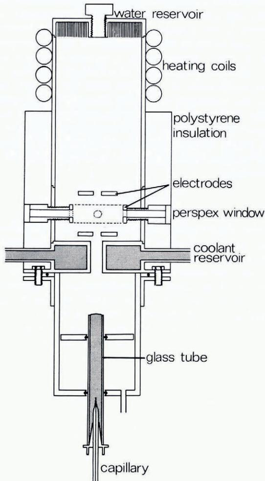
Fig. 1. Diagram of the drop production and suspension chambers.
