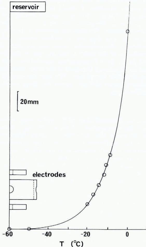
Fig. 2. Typical variation of vertical temperature gradient in the suspension chamber.
