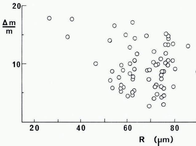
Fig. 5. Variation of measured values of percentage mass loss  $\Delta m/m$  as a function of drop radius  $R$ .
