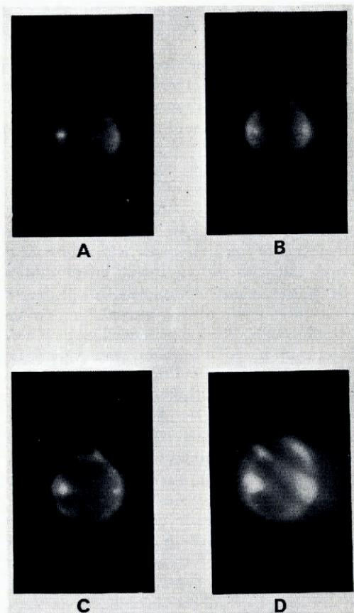
Fig. 3. Four frozen drops supported in the electrodynamic field, showing: A, approximate sphericity; B, slight bulge; C, large bulge; D, a drop which had apparently frozen along clearly defined planes. All the drops have a radius of approximately  $75 \mu\text{m}$ .
