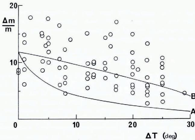
Fig. 4. Variation of the measured values of percentage mass loss,  $\Delta m/m$  with degree of supercooling  $\Delta T$ . Curve A is the calculated variation of evaporative mass loss for a drop in an environment of 90% relative humidity with respect to ice. Curve B is the maximum evaporative mass loss assuming no conduction between a drop and its environment.
