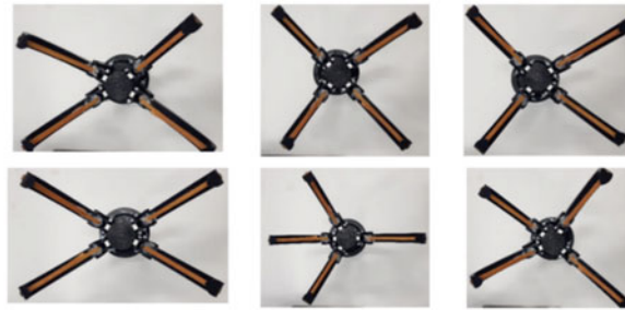
Figure 10. Top view of the robotic gripper in different configurations, shown in the opening state.
