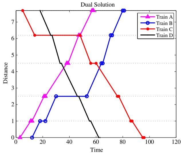
FIGURE 4. Four-train best dual solution with cost 98.920.
