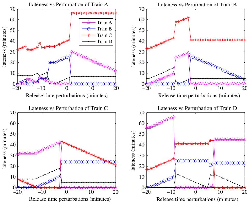
FIGURE 6. Variation in lateness versus release time of each train.
