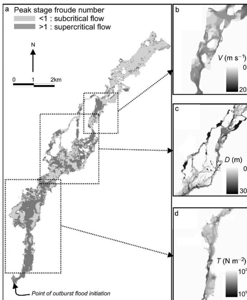
**Fig. 6.** Examples of 2D hydrodynamic model output and GIS-based calculations of (a) flow regime at peak stage after 2 hours, (b) flow velocity after 1 hr 30 min, (c) flow depth at peak stage and (d) shear stress after 1 hour. Note that diagrams do not necessarily pertain to the same model run, nor to the same hydrograph stage.
