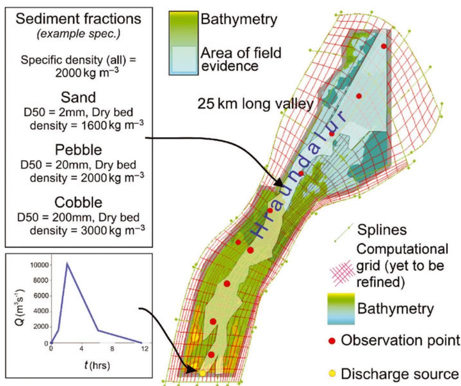
**Fig. 2.** Diagram of model input, illustrating bathymetric depth derived from a Digital Elevation Model (DEM) and computational orthogonal grid with a shape specified by user-defined splines. Flood input hydrograph and typical sediment fractions are also given. Sediment can be input with the hydrograph and pre-exist along the channel. Area of field evidence is after Carrivick and others (2004a).
