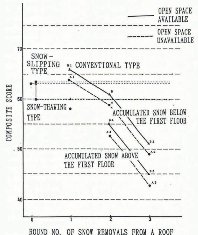
Fig. 6. Composite scores for snow removal from a house site.
