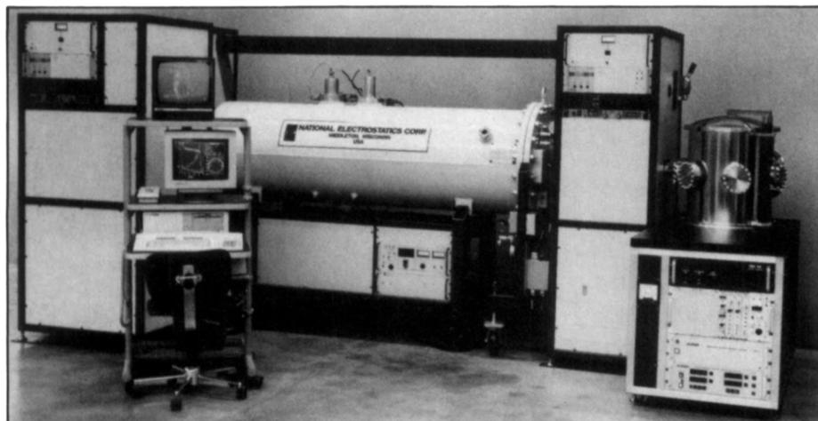
**MeV Ion Beam Surface Analyzer**
