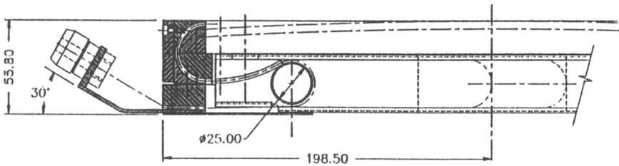
Figure 2. Cross-section of the southern half of one of the FLAIR II compact fibre plateholders, showing the fibre route around the edge of the field plate (uppermost in diagram) to the retraction storage loops behind. Dimensions are in mm.
