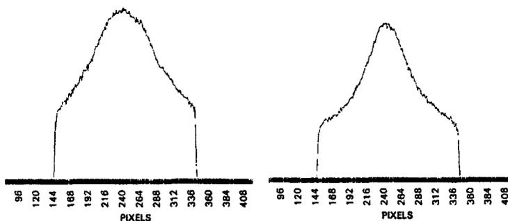
Figure 3. Output end intensity patterns when a  $153\ \mu\text{m}$  diameter fibre is centrally illuminated at its input end by a spot of about  $1/3$  its diameter (left) and  $1/10$  its diameter (right), showing highly-incomplete scrambling. Beam focal ratio  $f/2.8$ .
