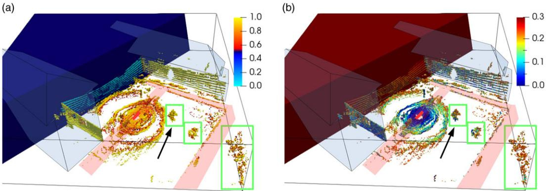
**Figure 12.** Reconstructed scene derived from lidar data (~320, 000 rays) using the proposed algorithm. Coloring is associated to the degree of occupancy value of the cells (i.e., most likely degree of occupancy left and standard deviation right).
