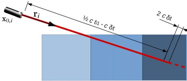
**Figure 7.** Schematic representation of lidar ray propagating in the new model parameter field  $\tilde{\mathbf{m}}(\mathbf{x}, t) = \{\tilde{\mathbf{m}}(K, t)\}_{K=1}^N$  (see Fig. 5).
