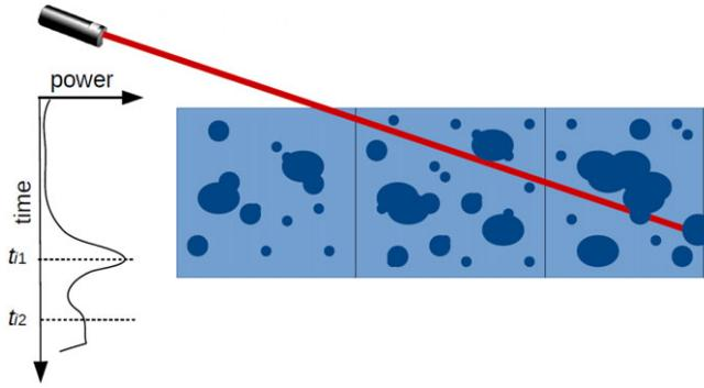
**Figure 5.** Schematic representation of lidar ray propagating in a scattering environment. Bins are associated to the spatial discretization  $\Omega = \cup_{K=1}^N \mathcal{V}_K$ . Recorded lidar power over time is indicated as well as the associated returned times as discussed in the text.
