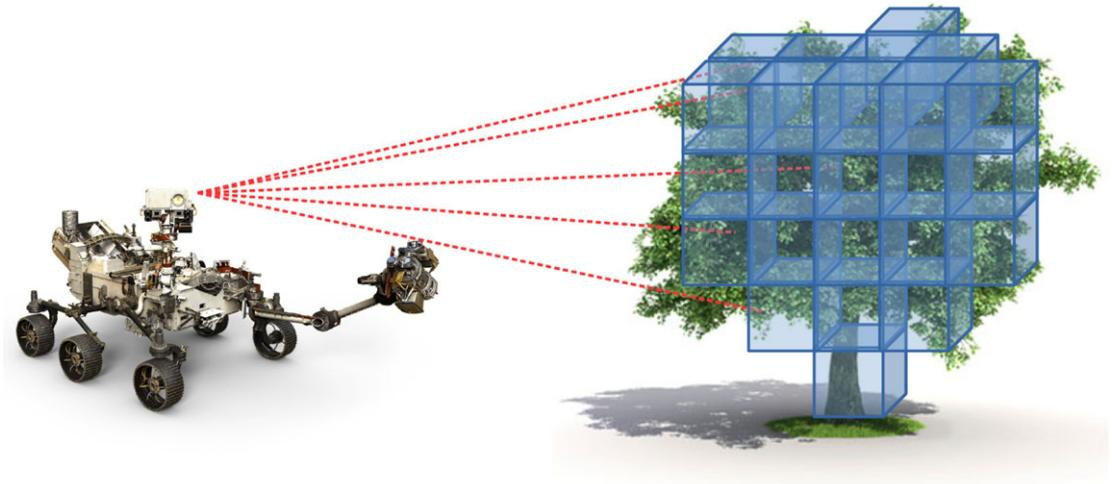
**Figure 1.** Schematic configuration of lidar data acquisition using a mobile robot. Red dotted lines represent lidar rays. The robot record time of flight is associated to each ray. Several voxels associated to the occupancy field discretization for mapping purpose are displayed in blue. Rover image credit: NASA/JPL–Caltech.
