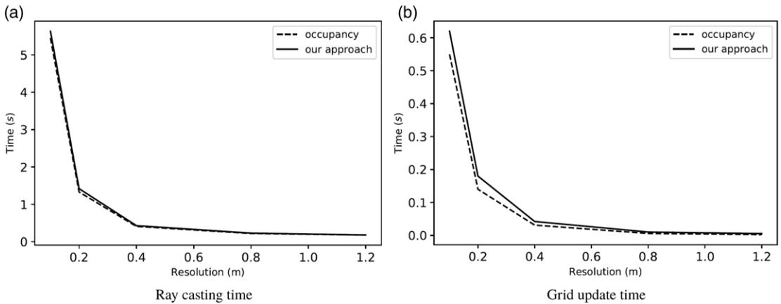
**Figure 14.** Run times associated to lidar data assimilation for different grid resolutions. (a) Ray casting time. (b) Grid update time.
