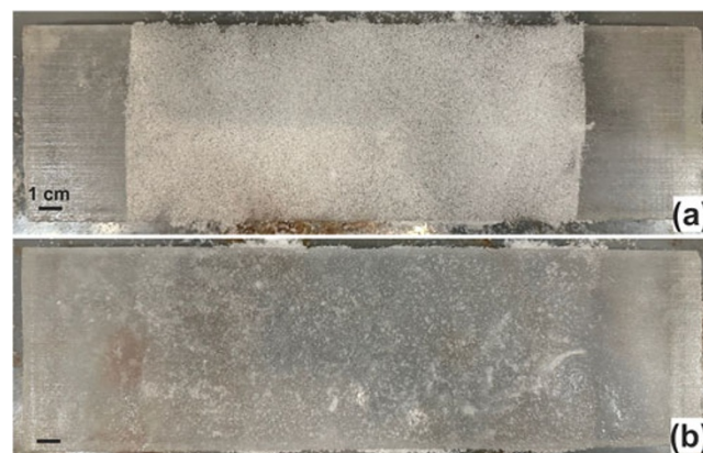
Figure 2. Photographs of a freshwater ice plate with a thin layer of freshwater ice fragments placed atop: (a) before spraying, and (b) after spraying with freshwater and consolidating the fragments through freezing.
