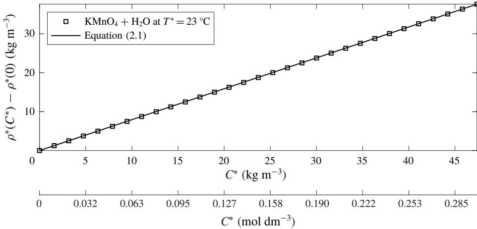
FIGURE 8. Density difference between aqueous solutions of  $\text{KMnO}_4$  and water (symbols) as a function of  $\text{KMnO}_4$  concentration at constant temperature ( $T^* = 23^\circ\text{C}$ ,  $\rho^*(0) = 997.54 \text{ kg m}^{-3}$ ). The linear function defined by (2.1) (solid line) approximates very well the correlation proposed by Novotný & Söhnel (1988) (symbols) in the range of values of interest.
