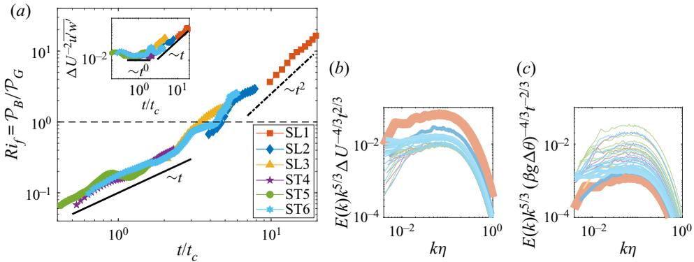
Figure 2. Temporal scalings of the turbulent kinetic energy: (a) ratio between the buoyancy and gradient  $ke$  production (i.e. the flux Richardson number  $Ri_f$ ) integrated over the wall-normal direction, with the inset showing the scaling of  $\overline{u'w'}$  at the centreline; energy spectra normalised with the (b) shear and (c) RT scalings for all the simulations (see (4.4)); the line thickness is proportional to the non-dimensional time.
