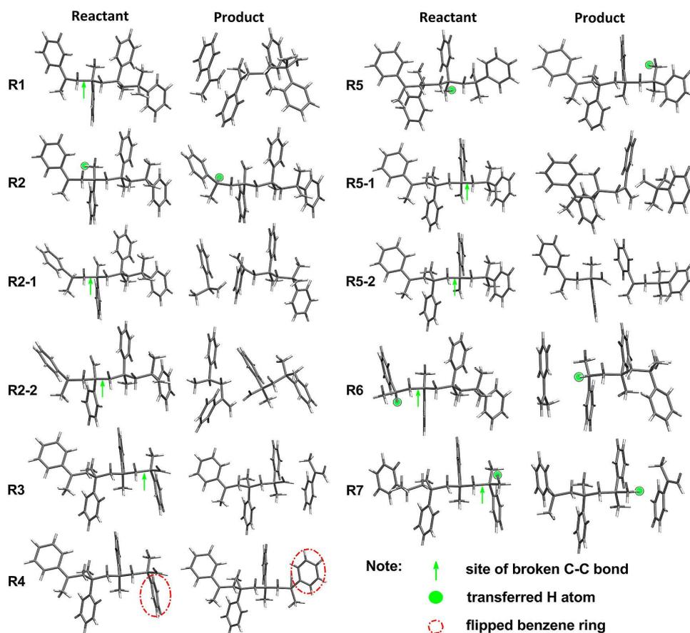
**Figure 2.** Geometric images before and after reactions. Here, the green arrows indicate the site of broken C–C bonds, and the green circles and red dash circles, respectively, denote the H atom and benzene ring involved in reactions.
