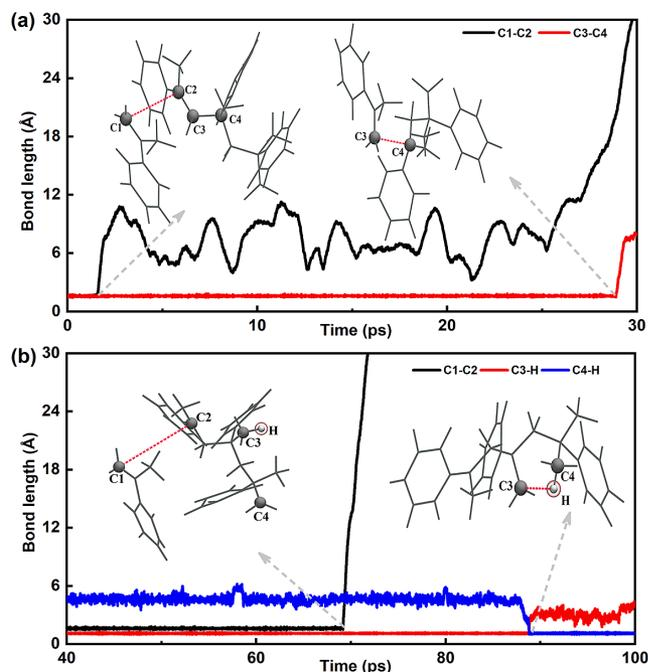
**Figure 3.** Dynamic simulations of the degradation processes of di-radical MM-PAMS at 550 K. These figures represent the bond length changes with respect to time for breaking sites on the backbone chain. Typical conformations during degradation are also drawn. C1–C2, C3–C4 and so on are the positions of broken bonds during degradation.
