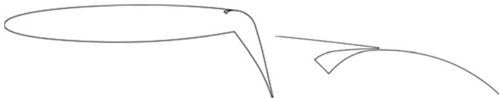
Figure 4. DLR F15 aerofoil with a 25% high-lift flap, deflected by 65°, and using internal blowing along a suited Coanda geometry as a reference (left) and blowing slot details (right).
