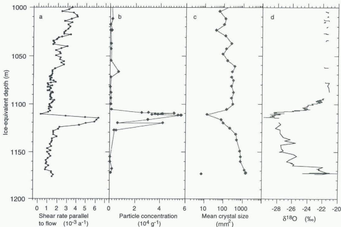
Fig. 2. Data around the shear-rate spike. Depths of the ice-core data are internally consistent but may have up to 4 m offset with respect to the shear-rate data.
