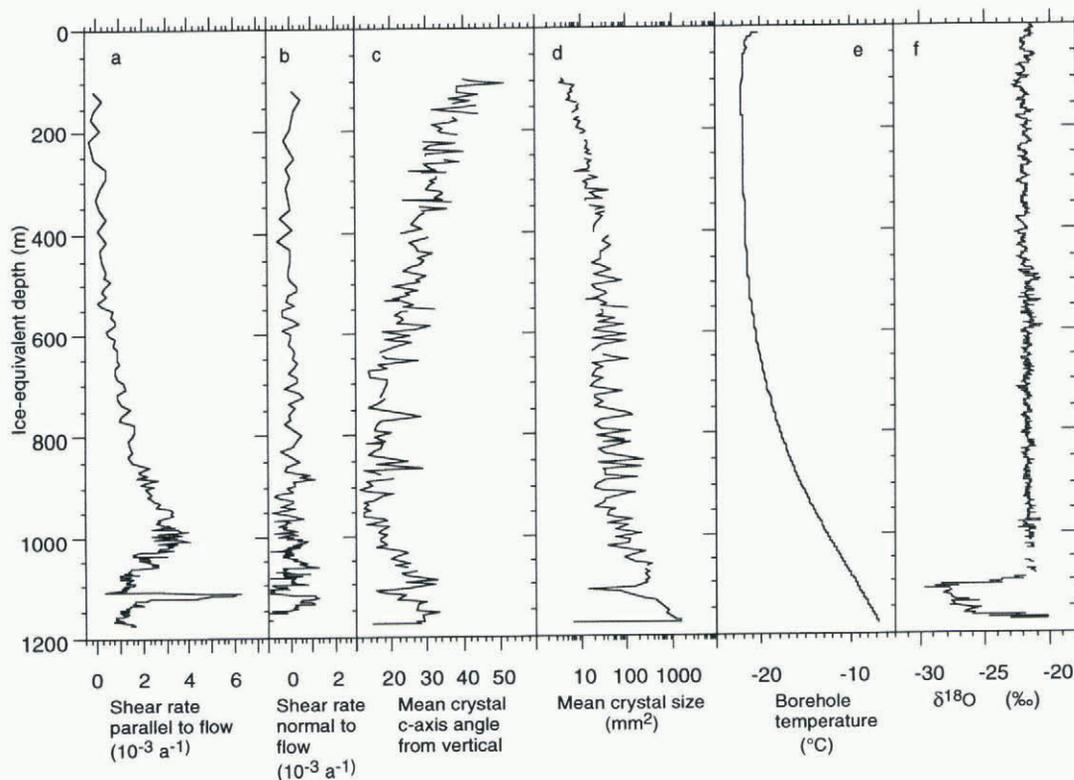
Fig. 1. Borehole and ice-core data. Depths are ice equivalent (adjusted assuming an equivalent ice thickness for the low-density firn in the top  $\sim 100$  m). (a, b) Shear rates projected on planes normal and parallel to the surface flow. (c, d) Data from crystal thin sections. About 100 crystals are measured for each section. (e) Measured temperature in the borehole. (f) Smoothed oxygen-isotope ratio with respect to Standard Mean Ocean Water.
