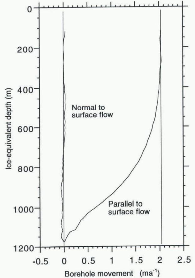
Fig. 3. Borehole movement obtained by integrating strain rate over depth.
