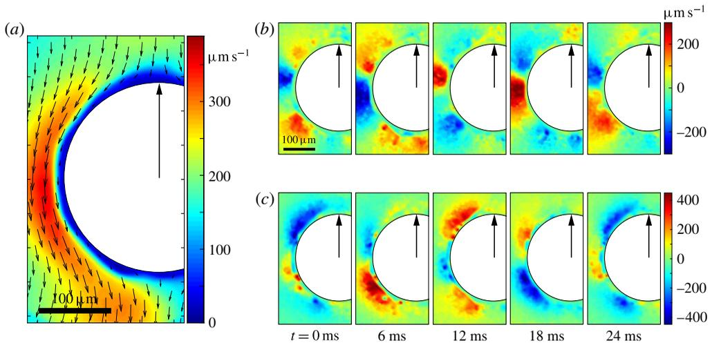
FIGURE 4. Experimental flow fields. (a) Magnitude (colour) and direction (arrows) of the time-averaged velocity field measured with PIV. Radial  $u'_r$  (b) and tangential  $u'_\theta$  (c) components of the unsteady fluid velocity field shown at various times through one flagellar beating cycle. Parts (a) and (b) are adapted from figures 1(c) and (d), respectively, of Brumley *et al.* (2015a).
