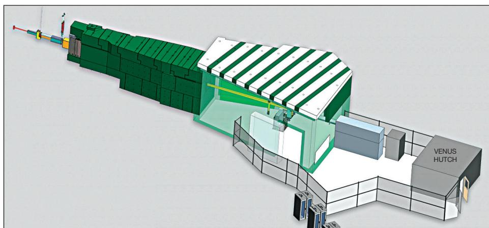
Schematic representation of the VENUS instrument, providing time-of-flight neutron imaging capabilities, at the US Department of Energy’s Oak Ridge National Laboratory (ORNL) in Tennessee. Credit: Jill Hemman, ORNL.
