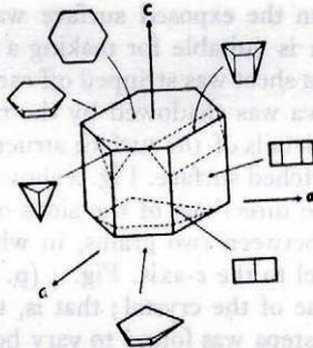
Fig. 1. Diagram to show the kinds of etch pits formed on ice
