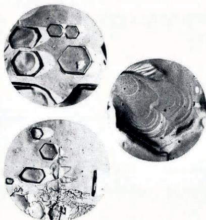
Figs. 2 and 3 (left). Microphotographs of shadowed replicas of etched ice crystals. The crystal in Fig. 2 and the grain on the left of Fig. 3 have faces perpendicular to the *c*-axis. The right hand grain in Fig. 3 has a face parallel to to the *c*-axis. Magnification  $\times 13$
