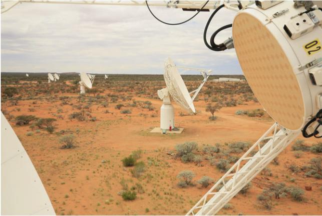
**Figure 1.** 12 m ASKAP antennas with PAFs at their foci at Inyarrimanha Ilgari Bundara, the CSIRO Murchison Radio-astronomy Observatory. Credit: CSIRO.
