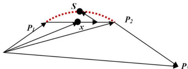
Scheme 1. (Color online) A very simple 3D-spline algorithm. Adding to point  $x$  the vector  $y = P_2 - P_3$ , scaled by spline parameter  $r$  leads to spline point  $S$ . One may also add an additional, small shift  $z = P_2 - P_1$ , scaled by the projection of  $r \cdot y$  onto  $z$ , as shown. However, the improvement is small because the angle  $P_1 - P_2 - P_3$  is around  $90^\circ$  for most helices.
