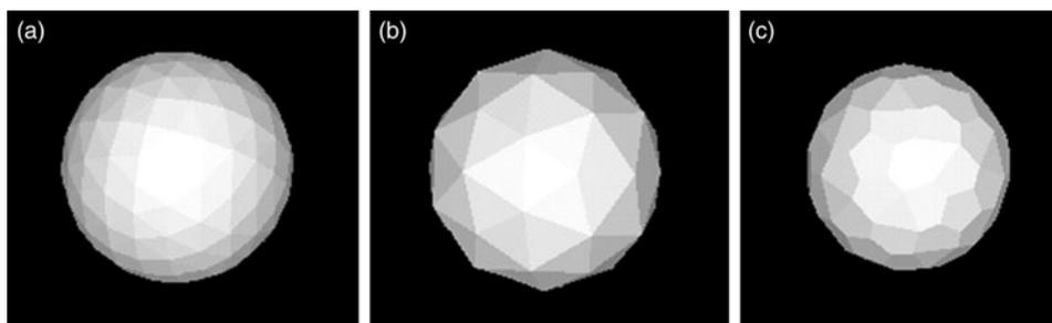
Figure 3. Rendering of 3D printed elements. (A) quasi-smooth sphere for carbon, hydrogen, and many other atoms. (B) Non-sphere representation of nitrogen, (C) non-sphere representation of oxygen.
