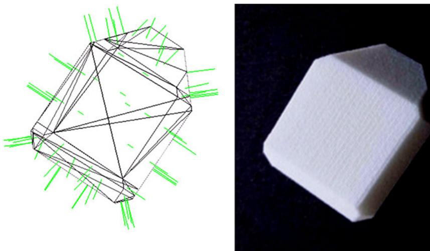
Figure 2. (Color online) Left: Screen-shot of a sugar (sucrose) morphology model with green lines representing the facet normal. Right: 3D printed model in nylon by the Selective Laser Sintering<sup>™</sup> (SLS<sup>®</sup>) technique, where the STL file was created from data in a CIF file with the WinXMorph software (Kaminsky, 2005, 2007). This model has dimensions of a few centimeters.
