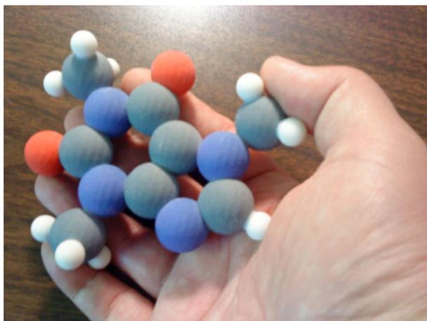
Figure 1. (Color online) 3D print of the caffeine molecule model [by the Color Jet Printing (CJP<sup>®</sup>) process].
