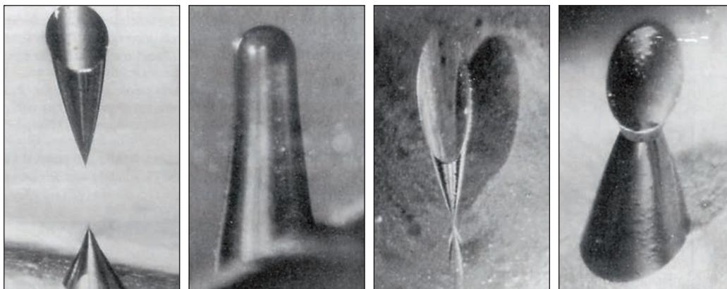
Etched tracks of cosmic rays that penetrated an Apollo 14 electrophoresis device that was made of Lexan. The taper and curvature of the tracks of the particles allow them to be individually identified. From left to right, argon, iron, calcium, and titanium ions. Credit: Springer Publishing Company.
