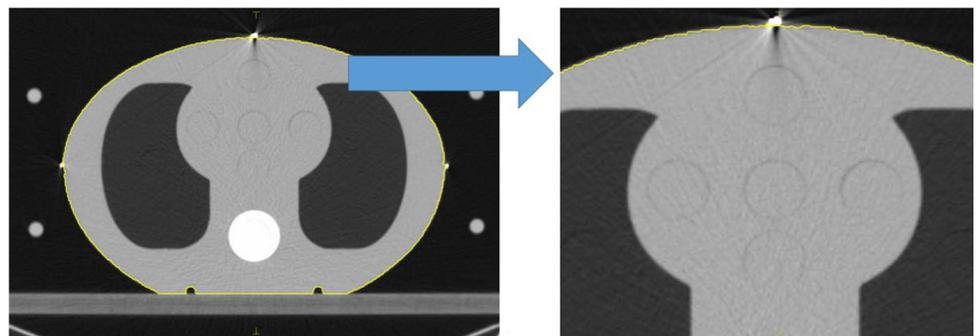
**Figure 2.** The fluctuations of external contour caused by automated tools.
