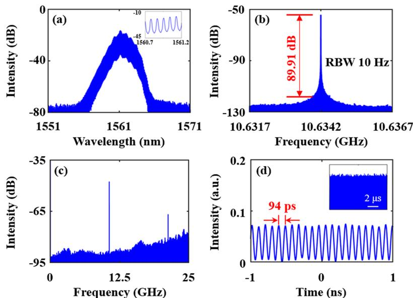
**Figure 4.** The characterization of the seed. (a) The optical spectrum. (b) The radio-frequency (RF) spectrum measured at a resolution bandwidth (RBW) of 10 Hz. (c) The RF spectrum measured at a 25-GHz span at an RBW of 30 kHz. (d) The oscilloscopic trace. Here, the pulse train at a 10.6-GHz repetition rate is viewed as a sinusoidal waveform due to the limitation of the electrical bandwidth. The inset shows the pulse trace in a wider span of 10  $\mu$ s.
