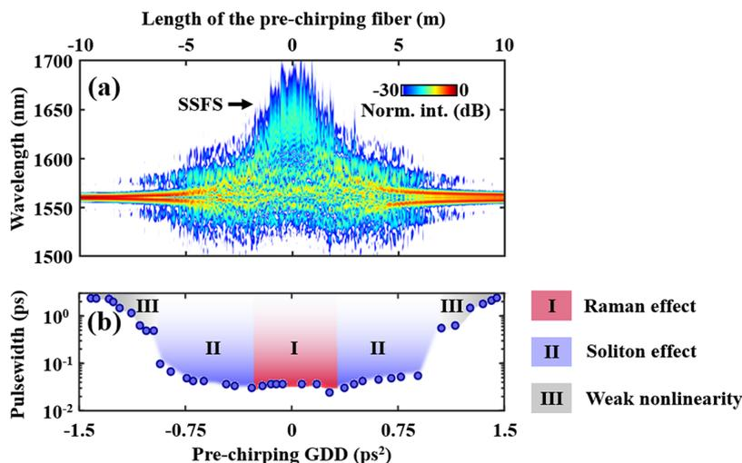
**Figure 2.** Numerical simulations of the amplified signals with different pre-chirping group delay dispersions (GDDs). (a) The contour plot of optical spectra with varying pre-chirping dispersion. SSFS, soliton self-frequency shift. (b) The corresponding pulsewidth variation. Regimes I, II and III are designated according to the spectral-temporal characteristics, and the pulse amplifications governed by the Raman effect, the soliton effect and weak nonlinearity, respectively, are identified.
