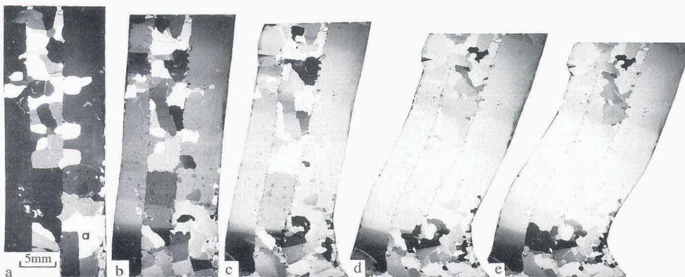
Fig. 5. The microstructural evolution in an anisotropic ice aggregate with non-axial shortening that involves a dextral shear of the sample (experiment BW 67). (a) Starting sample; (b–e) are 5%, 8%, 13% and 16% average longitudinal shortening strains, respectively.
