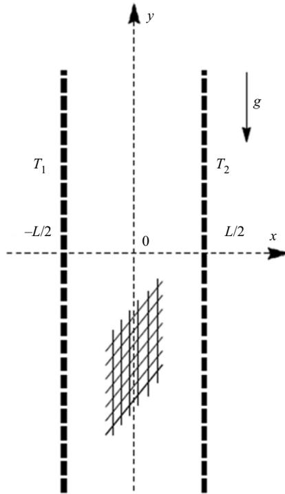
Figure 1. Schematic of a vertical porous slab.
