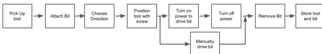
Figure 3: Example of user workflow in the context of a power screwdriver
