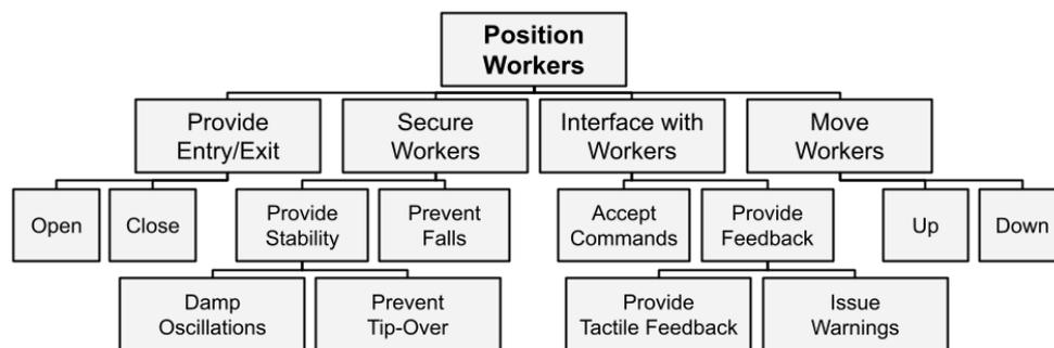
Figure 2: Example of function tree in context of articulating-boom construction lift
