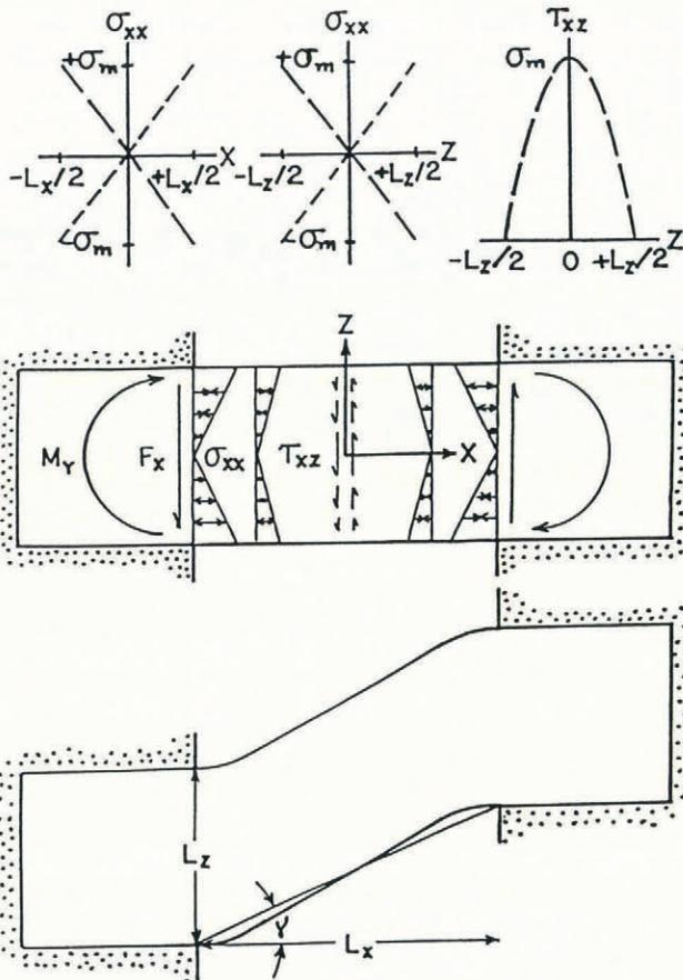
Fig. 6. Stresses and deformation of an ice specimen mounted in the simple shear-creep configuration shown in Figure 5. Top: the distribution of elastic shear stress  $\tau_{zx}$  and bending stress  $\sigma_{xx}$  in response to shear force  $F_x$  and bending moment  $M_y$  at the onset of creep deformation. Bottom: the distribution of viscoplastic shear and bending produced by strain  $\gamma$  at the conclusion of creep deformation. Bending is suppressed when  $L_x \ll L_z$ .
