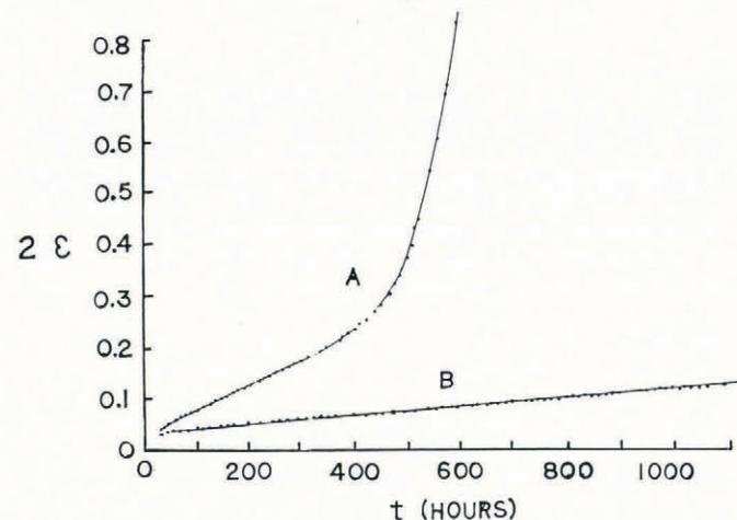
Fig. 7. Creep curves for simple shear of laboratory polycrystalline ice conducted at  $-3^\circ\text{C}$  using the creep configuration in Figure 5 to duplicate the shear bands in the calving ice wall on Deception Island. Curve A:  $\tau_{zx} = 117$  kPa; curve B:  $\tau_{zx} = 55$  kPa.
