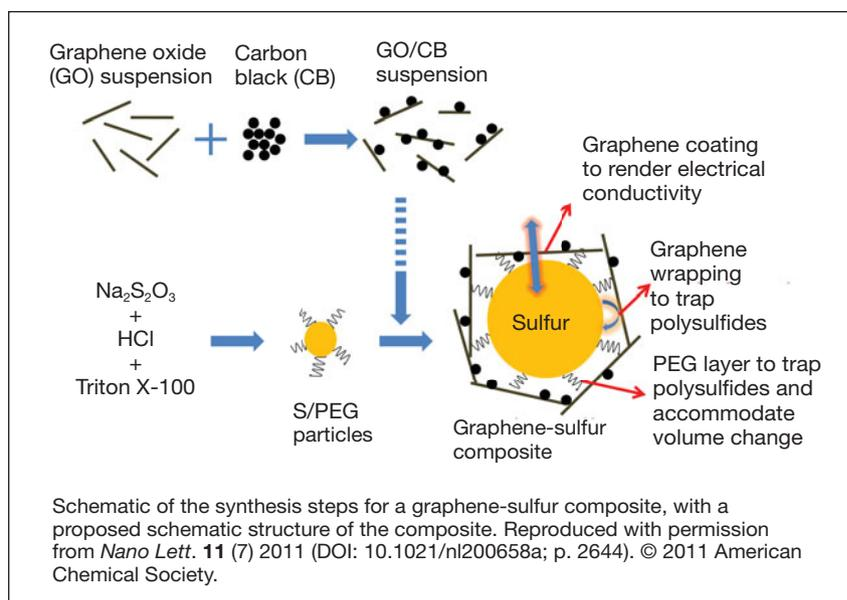
intermediates and rendering the sulfur particles electrically conducting. The team found that the average size of the sulfur particles was less than 1  $\mu\text{m}$  and energy dispersive spectroscopy was used to confirm the structure and composition of the graphene-sulfur composite. Colorimetric titration experiments determined that the graphene-sulfur composition contained 70 wt% of sulfur (with 15% of mildly oxidized graphene sheets and 8% carbon black).
