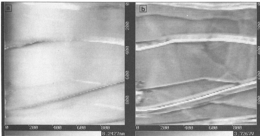
(a) Surface boundaries of highly oriented pirographite are visible on the surface AFM topography image. (b) Using UFM reveals additional subsurface grain boundaries.
