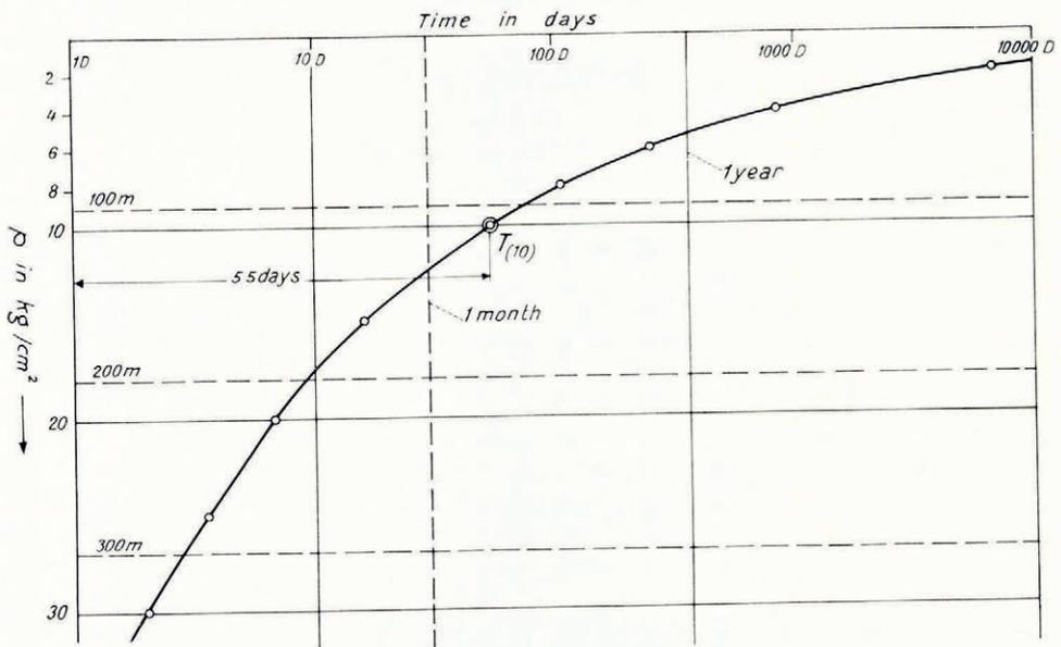
Fig. 13. Half-life curve of the closing process of a vertical cylindrical shaft, as a function of the overburden pressure or the depth, for temperate ice.
