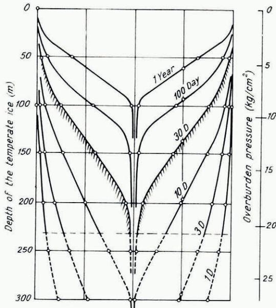
Fig. 14. Different stages of the closing process of a vertical cylindrical shaft in temperate ice.
