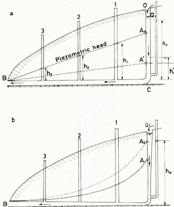
Fig. 15. Simplified hydraulic model (schematic) for water circulation in a glacier snout (temperate ice).
