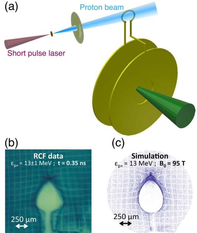
**Figure 6.** Example of a proton deflectometry measurement: (a) schematic of the setup; (b) image obtained on RCF with 13 MeV protons; (c) simulation of proton deflection in a  $B$ -field<sup>[35]</sup>.
