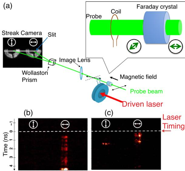
**Figure 5.** Example of a Faraday rotation measurement: (a) typical setup; (b) reference image; (c) image in the presence of a  $B$ -field<sup>[32]</sup>.
