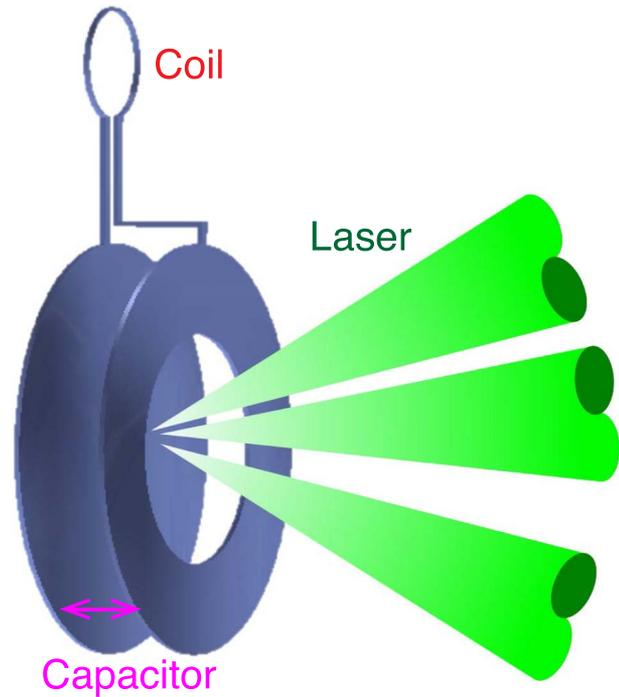
**Figure 1.** Basic geometry of the capacitor–coil target.
