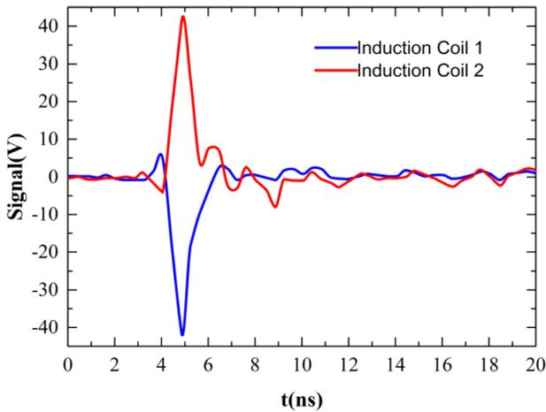
**Figure 4.** Typical symmetric signal observed with a differential twisted pair<sup>[38]</sup>.
