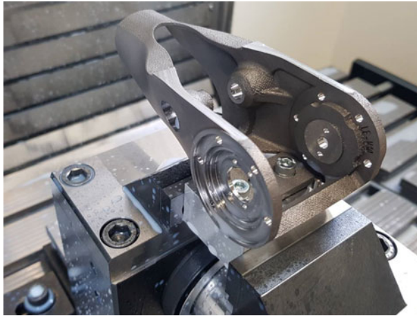
Figure 7. Machining of the 3D-printed titanium knee-interface element.
