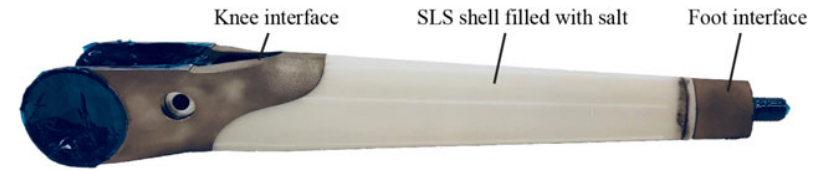
a) Pre-assembled shell with SLM parts
