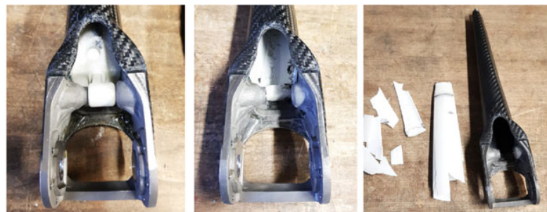
e) Tool removal: Drilling through shell, salt removal and mechanical removal of shell
