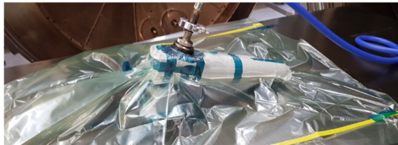
d) Vacuum bagging and autoclave curing
