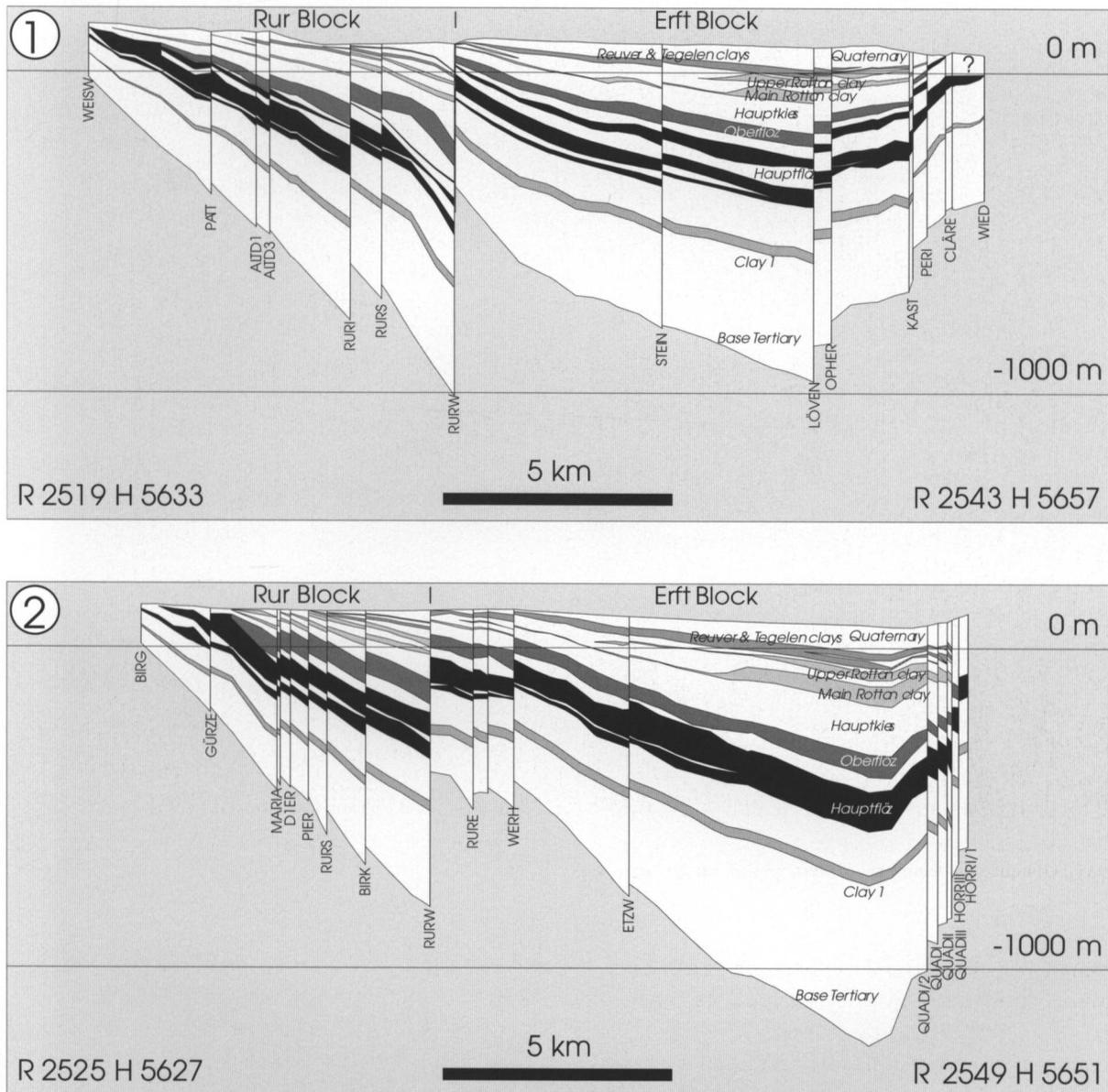
Fig. 9. Two southwest-northeast striking cross-sections through the Rur and Erft Blocks. For location of these sections refer to Fig. 1; vertical exaggeration 10:1.
