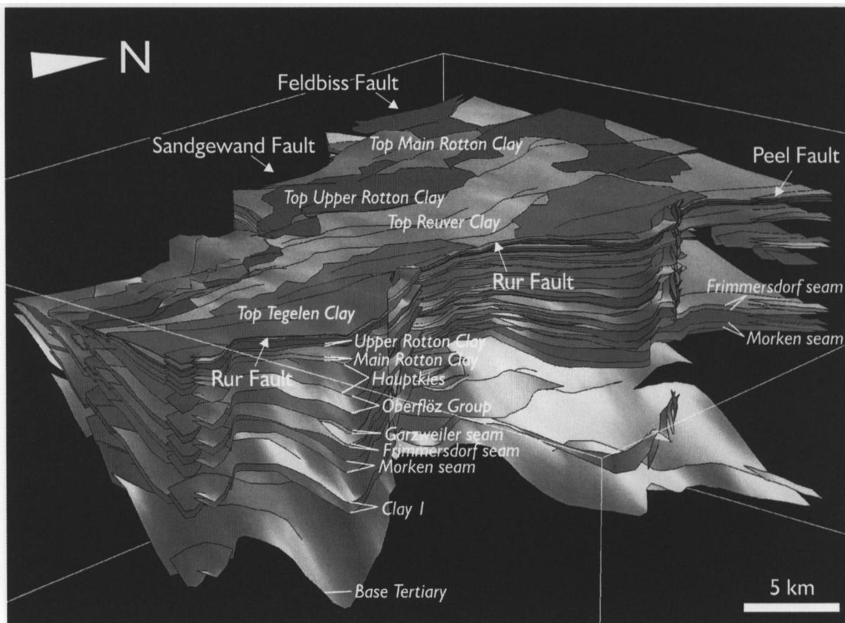
Fig. 8. GOCAD model of the Rur-Block made up of 20 stratigraphic surfaces ranging from Base Tertiary to the Reuver and Tegelen clays (Hager, 1981). Oblique view from East to West; vertical exaggeration 10:1.
