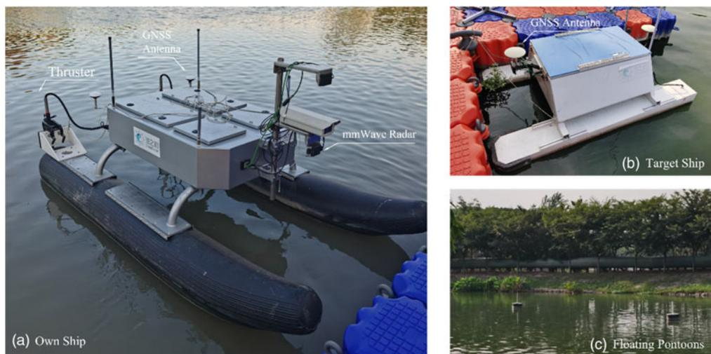
**Figure 7.** Sketch of the experimental system, including the own ship (a), the remote-controlled vehicle (b) and the floating pontoons with diameter of 0.9 m (c).
