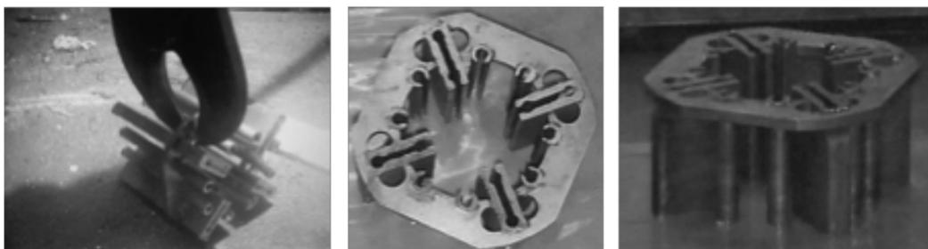
Figure 3 Pictures taken underwater showing the final item to test in release rate analysis.
