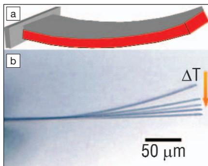
Figure 1. (a) Schematic illustration of a bimaterial cantilever bending with incident heat. (b) Side view of an optical image of a polymer-silicon microcantilever bending as the temperature increases 20–40°C. Reproduced with permission from *Nano Letters* 6 (4) (April 12, 2006) p. 730; DOI: 10.1021/nl0525305. © 2006 American Chemical Society.
