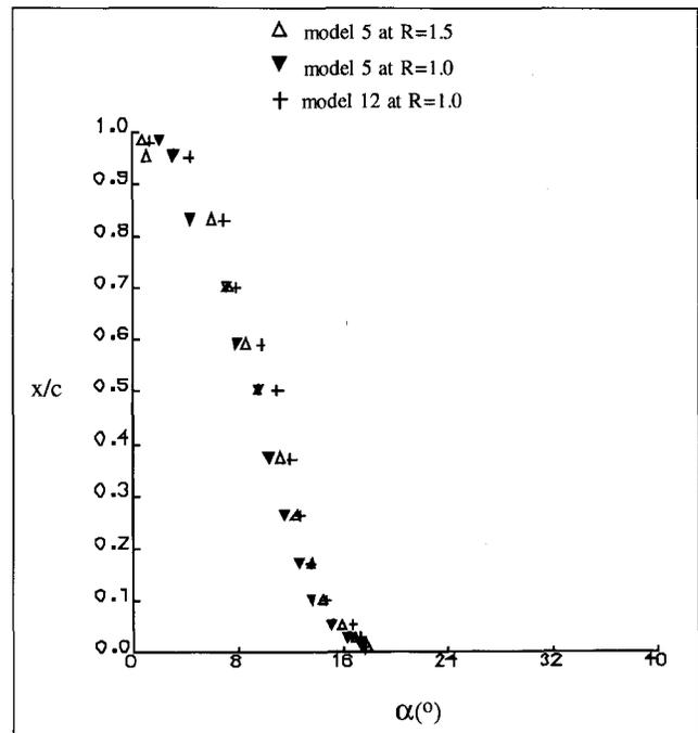
Figure 11. Reattachment loci for ramp-down motion at  $r = -0.016$ . Model 5 at  $R = 1.5$  and  $R = 1.0$  and model 12 at  $R = 1.0$ .
