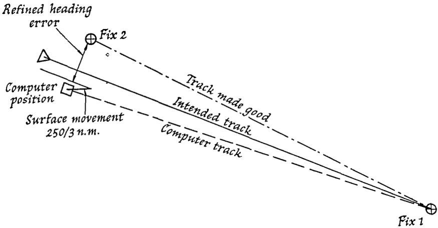
FIG. 2. Determination of heading error when sea movement is present
