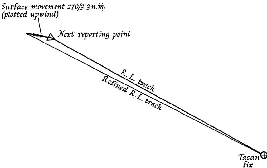
FIG. 3. Determination of refined R.L. track
