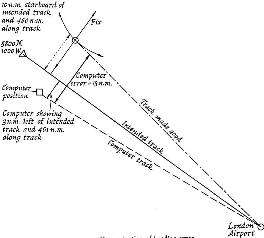
FIG. 1. Determination of heading error
